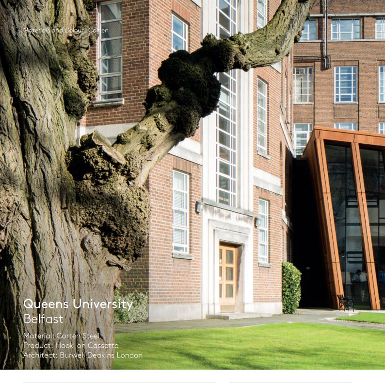
Corten Steel Façade option is a weathering steel façade that naturally rusts over time, producing a striking oxide finish. The rust creates a protective coating that constantly forms allowing the façade to self heal, creating a highly durable and low maintenance option.
