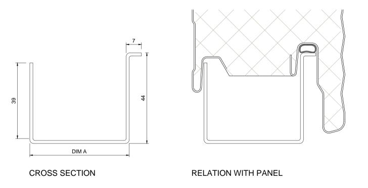
NOTE : ABOVE DIMENSIONS ARE THEORETICAL, ACTUAL DIMENSIONS WILL VARY DUE TO MANUFACTURING TOLERANCES. ALL DIMENSIONS ABOVE ARE IN MILLIMETRES. BASE CHANNEL FIXED AT MAX 500MM CENTRES AS SHOWN ABOVE. BASE CHANNEL TO BE CONTINUOUS AND SILICONE SEALED WHERE JOINTED. MATERIAL : 1.6MM THICK GALVANIZED STEEL
