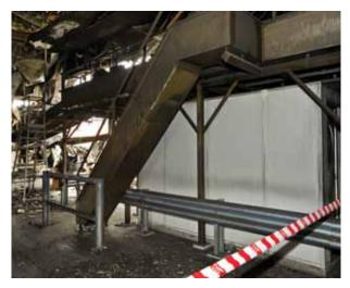
Kingspan PIR insulated panels remain unscathed after a major fire at a meat processing plant in 2010. Adjacent panels in EPS polystyrene (from another manufacturer) were incinerated.
