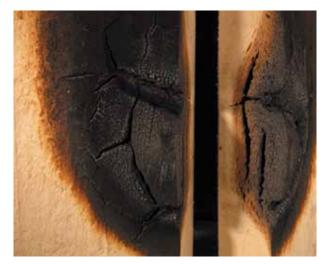
Section cut through the Kingspan PIR panel showing no fire propagation after 30 minutes
