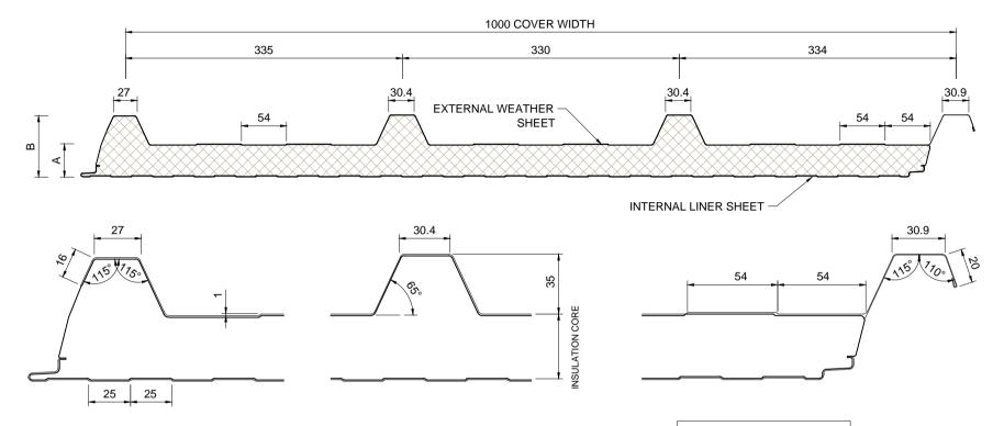
NOTE: ABOVE DIMENSIONS ARE NOMINAL, ACTUAL DIMENSIONS WILL VARY DUE TO MANUFACTURING TOLERANCES. EXACT DIMENSIONS MUST ALWAYS BE MEASURED FROM ACTUAL SAMPLES. ALL DIMENSIONS IN MILLIMETRES.
